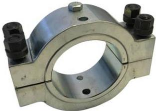
The first 5 sizes fit straight into the CLAMP and are retained with an M8 bolt in each half of the CLAMP as can be seen in the next picture. The SHELL sleeve shown is the largest of the set with a 75mm internal dimension. This SHELL sleeve also acts as a spacer sleeve for the 4 smaller sizes of SHELL sleeve.
