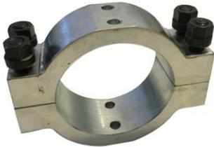
The picture on the left shows the outer form of the CLAMP system. The CLAMP is in 2 halves and is closed together around the bush using the 4 x 10mm studs & nuts. This ensures a high degree of compression around the full circumference of the bush without the risk of damage during the insertion process.
