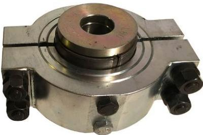
Clamp with No 1 SHELLS (75mm dia) & No 6 SHELLS (63mm dia) fitted and DAF bush in place ready for insertion. Note the tool will be set up from new in this configuration, this is to ensure all component parts are present and in position.
