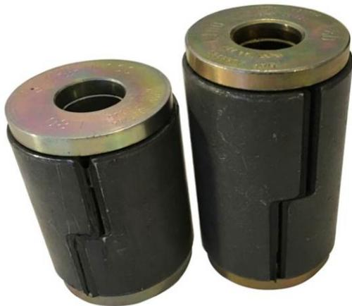
The 2 bushes in the picture are typical of the design and are both used in DAF tipper trucks where there may be more than 20 such bushes used throughout the suspension system. At each annual MOT safety check the condition of these bushes is carefully checked and if any wear is found then these must be replaced before the vehicle can be allowed back on the public roads.
