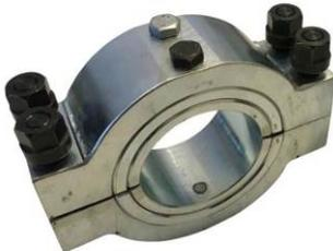
The next picture shows the first of the smaller SHELL sleeve bolted into place which takes the internal diameter down to 63mm. This is the size used by DAF on their bushes.
