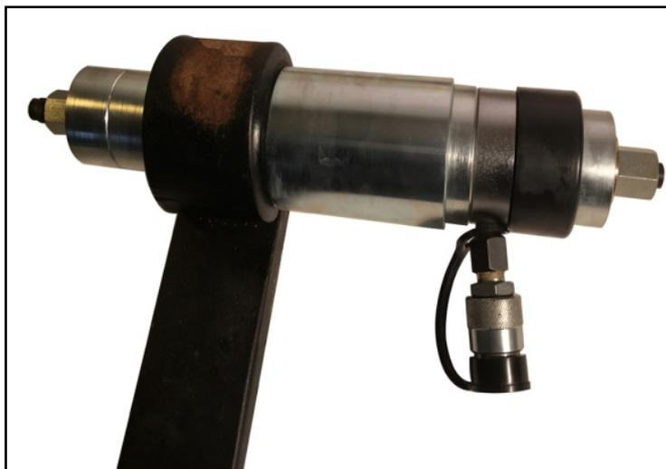
The old bush is gradually pushed out of the spring eye and is retained in the hollow receiver tube when clear of the spring. Despite the limited travel offered by this compact ram the removal is very quick using the adjustment nuts at each end of the DRAW ROD. The benefit of the compact ram is the limited space needed to operate. This more than compensates for the limited travel on each stroke of the ram.
