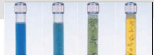
A strong colour change from blue to yellow, using either the standard or sensitive reaction fluid, indicates the presence of carbon dioxide in a vehicle's cooling system.
