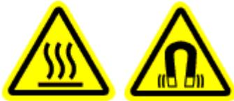
Do not wear clothing that is made with metallic pocket rivets, waist band buttons, pocket buttons, and zippers when operating the Mini-Ductor® Venom™. The Mini-Ductor® Venom™ can heat such metallic items very quickly and cause serious burns or even ignite clothing.
