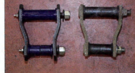
New and old shackles – note the grease nipples on the pin ends
